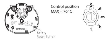
25) IMPORTANT: It may be necessary to remove the element to ensure correct engagement of the thermostat terminals to the element terminals
