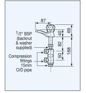
This tap is constructed to control the flow of incoming mains water supply to an open outlet type electric water heater. This displaces the heated water in an unrestricted flow through the tap's permanently open outlet. This vented hot tap is for full bore plumbing.
