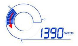
When the gauge moves in the direction of red arrow, your household is taking energy from the grid and the amount of power taken is shown.
