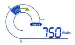
When the gauge moves in the direction of green arrow and the export symbol is shown, your household is generating more power than it is using and therefore exporting some power onto the grid. The value of energy available to use is shown in Watts. The Solar iBoost+ will be diverting energy to your immersion heater unless the tank is hot.
