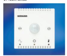
The S1 can be used with any Heatrae Sadia Aerheat heater and offers the benefit of potential energy savings and improved comfort. Once activated from up to 5 metres the controller allows the heater to increase the room temperature to its designated comfort setting of between 19°C to 25°C. If no movement is detected within a predetermined time (between 30 mins to 3 hours) the heater is switched off or the temperature can be held at a lower background level of between 0°C and 17°C.
